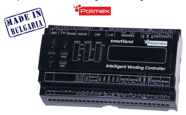
**ICON 180 SMARTVEND**Specialized controller for management of vending machines, which replaces the embedded money mechanism and eliminates the need of cash register. It uses standard EXECUTIVE protocol. That is why it can work with most of the vending machines.
