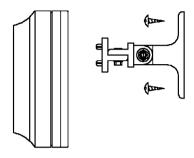
2. Attach the Camera Case to the bracket.
