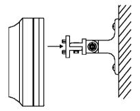
3. Adjust the vertical and horizontal angles by loosening screws (A&B) and by turning the bracket vertically and horizontally.
